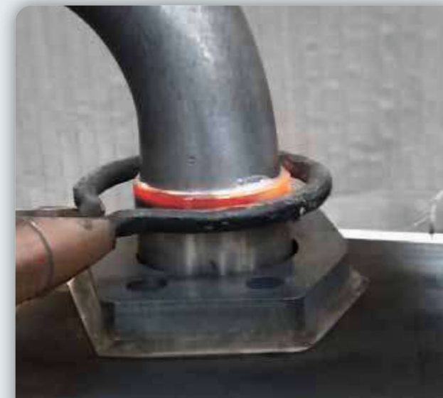
BRAZING STEEL ELBOW - BRASAGE COUDE ACIER Inductor L180/D120 Powerduction 160LG
