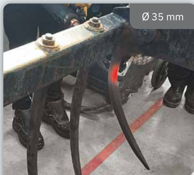
BUCKET TOOTH STRAIGHTENING - REDRESSAGE DENT DE GODET Inductor L20/B4 Powerduction 110LG
