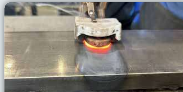
HEAVY METALWORK 20 MM STEEL - CHAUDRONNERIE LOURDE 20 MM Inductor L20/B4 Powerduction 220LG
