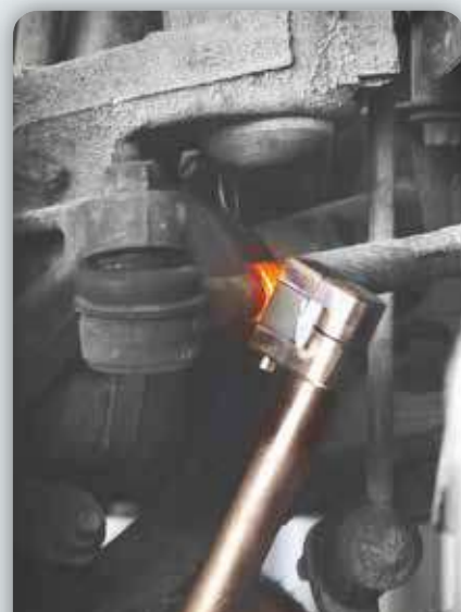
RELEASING CONNECTING RODS - DÉGRIPPAGE BIELLETTE DE DIRECTION Inductor S90 Powerduction 37L
