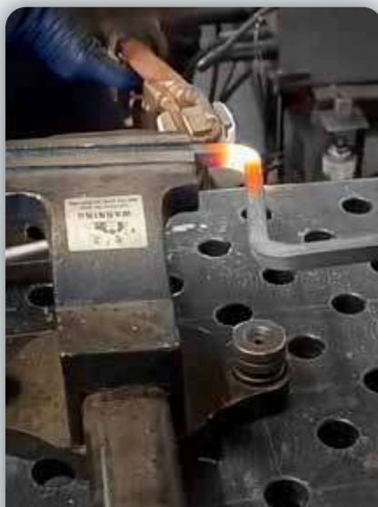
STEEL BAR BENDING - CINTRAGE BARRE ACIER Inductor L20/B4 Powerduction 110LG
