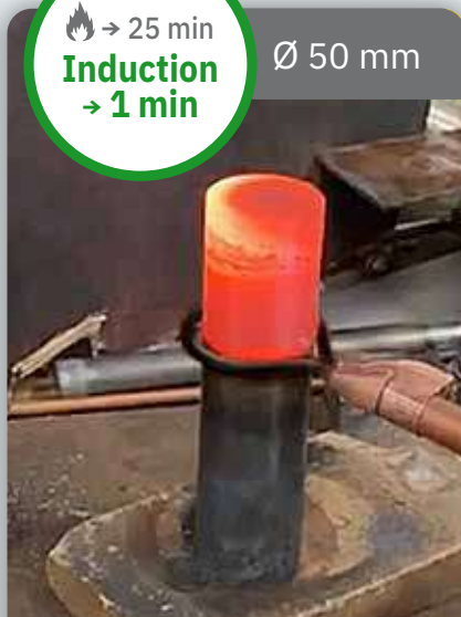
STEEL BAR FORGING - FORGEAGE BARRE ACIER Inductor L180/D60 Powerduction 220LG
