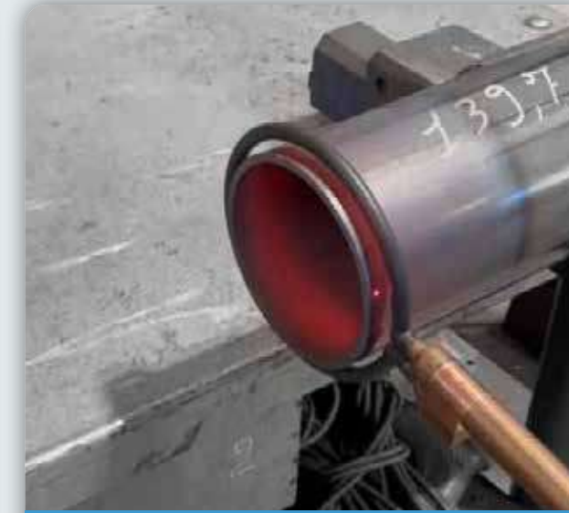
STEEL PIPE ASSEMBLY - EMBOITAGE TUBES ACIER Inductor L180/D150 Powerduction 160LG
