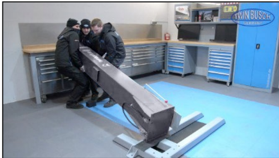
Illustration: Erecting the column
