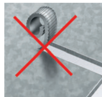
Notching without chip breaking
