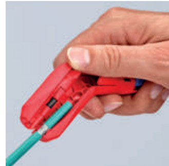
Stripping of a data cable
