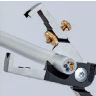
Induction-hardened shear blade with precisely ground cutting edges for crush-free cutting of copper and aluminium cables of up to Ø 15 mm (5 x 2.5 mm²)
