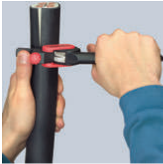
Turning the tool for circumferential cut
