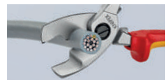
Final cut: after cutting the sheath in the front profile the conductors in the rear part are cut. Initial cut in the front profile, final cut in the rear profile – to keep it as easy as possible.
