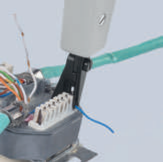
Inserts and cuts cables in one operation
