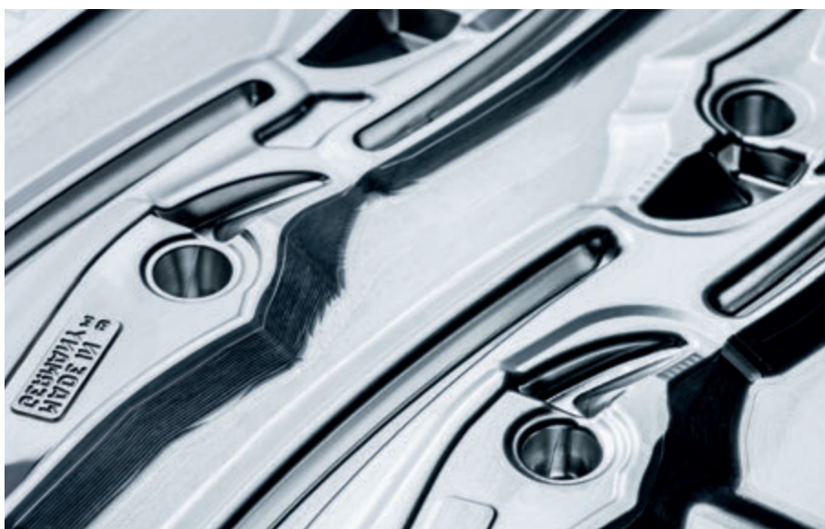
Forging die for the high leverage diagonal cutters with forged-in axle.
