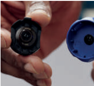
A spare cutting wheel is stored in the blue handle for quick replacement
