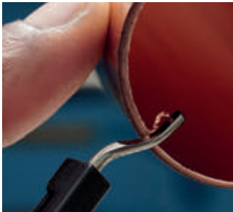
The precisely ground deburring tool can be taken out of the tool when needed.
