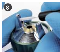
Clean the horn holes with special tiny brush (code W2COM6127).*
