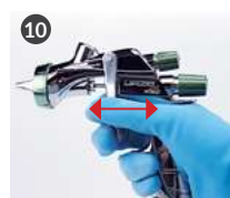
Check if the trigger and the needle travel smoothly.
