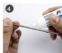
Grease the needle (code W2COM6165).
