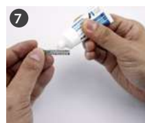
Grease the Needle spring.
