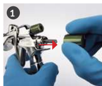
Take out the fluid adj. knob and needle spring.
