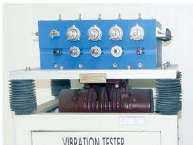
Vibration tests demonstrate the high impact resistance.
