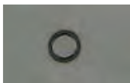
Inverter Spot HSS Steel 1,7+1,4+0,75 mm
