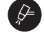
Pressing this key, the air continues to exit the torch for a pre-established time of approx. 20 sec (allows cooling of the torch and/or air adjustment within the optimal range).
