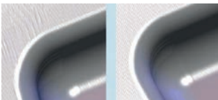
Perfect surface quality through reproducible results in adjacent milling paths (right picture)
