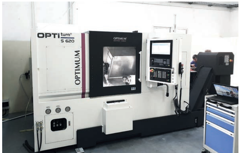
OPTIMUM PREMIUM CNC-Slant bed lathe S 620 with counter spindle
