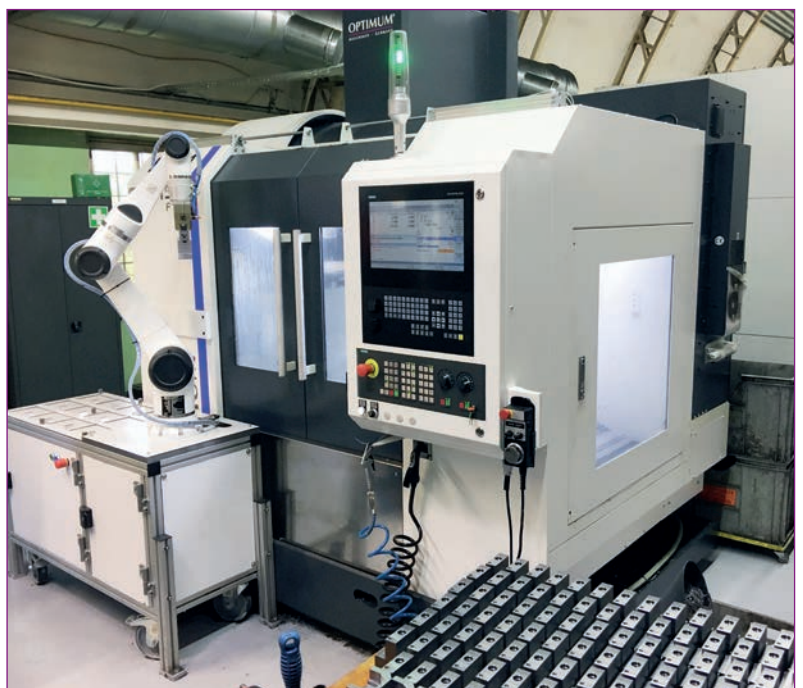
OPTIMUM CNC machines coupled to robots
