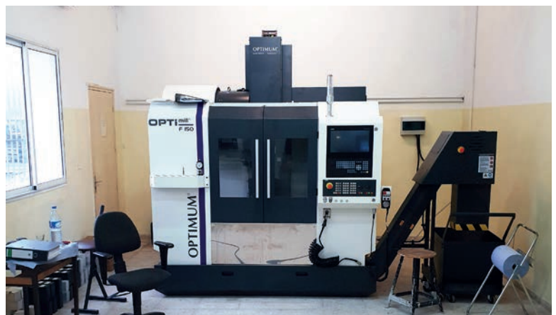
Three-axis OPTIMUM PREMIUM F150 HSC milling machine
