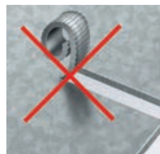
Notching without chip breaking
