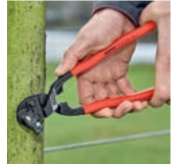
Two-hand operation for maximum cutting force
