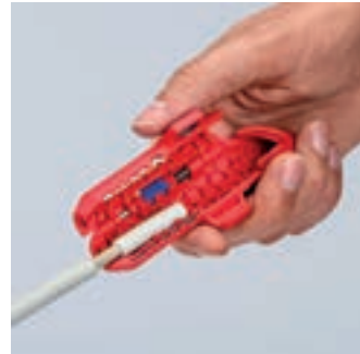
Stripping of a NYM cable
