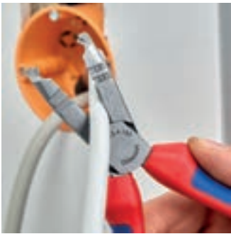
Cutting cable up to Ø 13 mm
